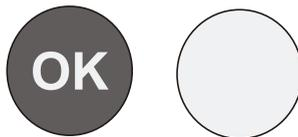
If the indicator of temperature turns WHITE, this means that the temperature is too high; in this case, increase the refrigerator temperature control setting and wait for 12 hours before performing a new visual inspection of the indicator. When fresh food has been introduced or the door has been left open, it is possible for the indicator of temperature to turn WHITE after a while.
